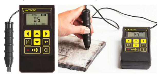
Crack depth meter TQ 281M – high-precision instrument for measuring the depth of cracks exposed on various metals and alloys (incl. stainless steel, duraluminum), previously detected by other methods.
