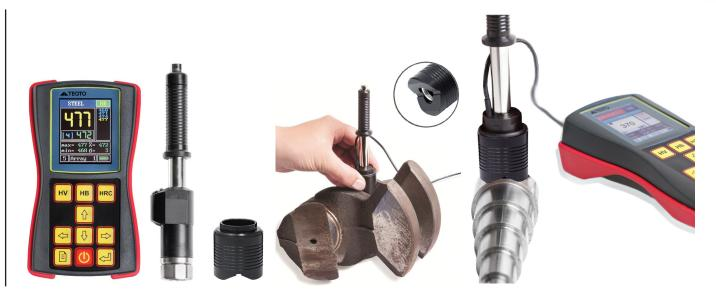
TQ Leeb Hardness tester TQ TKM-359CE special is successfully used in particularly difficult production and field conditions. Device is intended for non-destructive testing of production quality in metallurgy, mechanical engineering, aircraft, shipbuilding, atomic industry, oil and gas industry.
