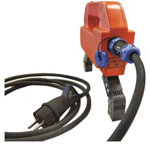
The AC electromagnetic yoke is suitable for magnetic particle inspection to detect surface and subsurface defects such as cracks, hair lines and tears of base material as well as incomplete fusion of welded joints.
