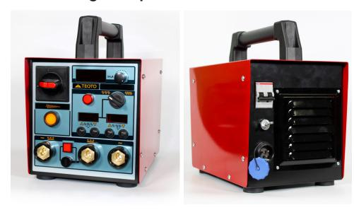
TQ STREAM-10 portable magnetic particle flaw detector is designed to detect surface and subsurface defects when testing products made of ferromagnetic materials. Incomplete fusion, cracks, and flocks can be identified.
