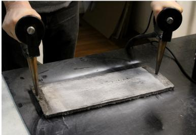
TQ STREAM-15 portable magnetic particle flaw detector is designed to detect surface and subsurface defects when testing products made of ferromagnetic materials. Incomplete fusion, cracks, and flocks can be identified.
