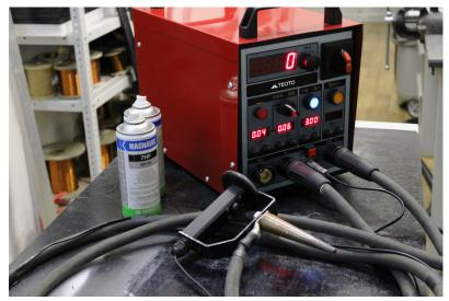
TQ STREAM-20 portable magnetic particle flaw detector is designed to detect surface and subsurface defects when testing products made of ferromagnetic materials. Incomplete fusion, cracks, and flocks can be identified.
