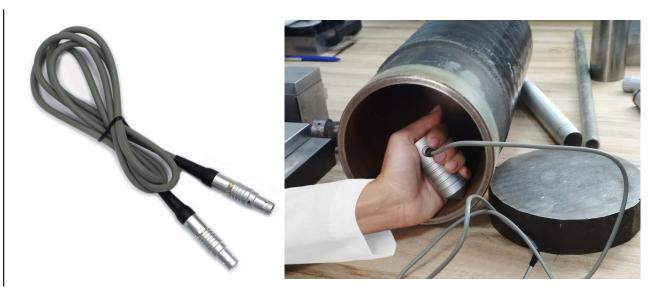
This cable is purposed to connect the electronic unit of the hardness tester TKM-459CE with a UCI probe. Connection cable suitable for probes:
