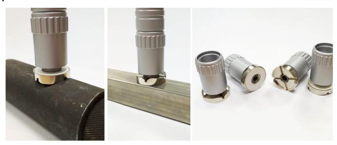
**Special head «U-459»** for positioning of probe on flat, curved, cylindrical surfaces. Minimum diameter of controlled item is 4 mm.
