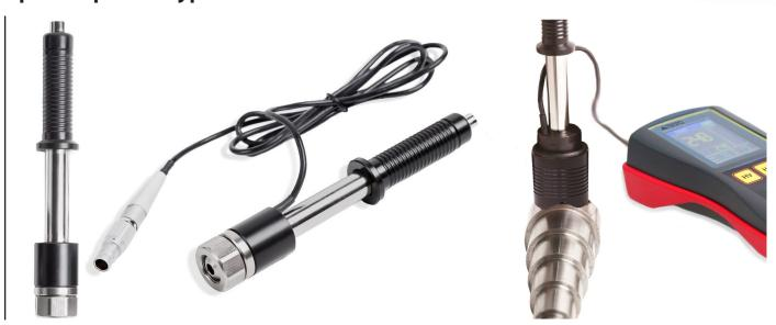
Special probe Type «E» is a replaceable probe for Leeb Hardness tester TQ TKM-359CE. Probe with indenter made of polycrystalline of boron nitride intended for control of materials with high hardness.
