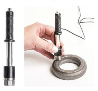
Standard probe Type «D» is included in the Basic delivery set of the Leeb Hardness tester TQ TKM-359CE
